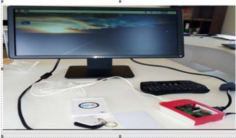
Figure 6.3.1 Physical Connection of Raspberry pi with Universal Serial Bus(USB) Near the Field Communication (NFC) Reader
