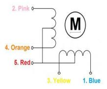
It should be noted that it is a 5V Stepper motor since the Red wire energize with 5V. It is a four phase stepper motor since it has four coils in it. Now, the gear ratio is given to be 1:64. This means the shaft that seen outside makes one complete rotation only if the motor inside rotates for 64 times. This is because of the gears that are connected between the motor and output shaft, these gears help in increasing the torque.
