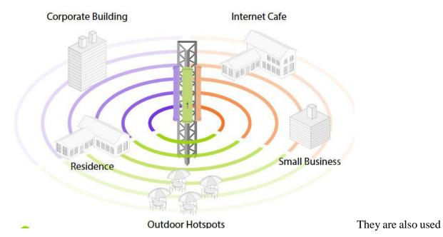
for other types of mobile communications, for example in Wi-Fi networks. They are used for limited-range distances of around 4 to 5 km.
