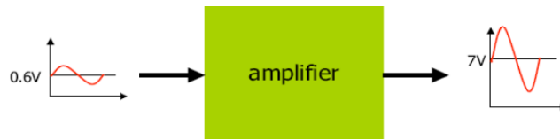
Fig 2.2 Symbol of transistor amplification
